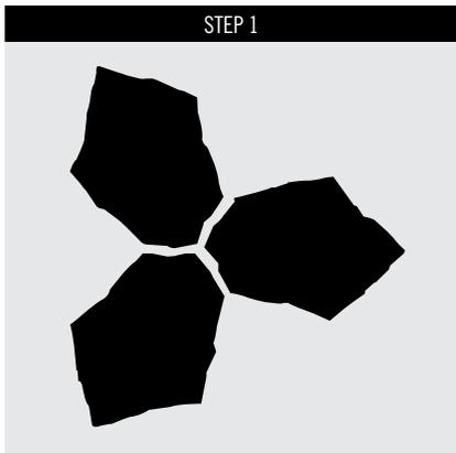
Begin by laying 3 pavers at the center of the surface to be covered.
